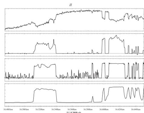
An example of time series of the laser altimeter and the line scan recording. The upper graph shows the distance between aircraft and local surface, including the vertical motion of the aircraft and the surface structure. The surface height (2nd graph from top) is computed from the distance subtracting aircraft height measured with the inertial navigation system of Polar 2. A high echo-intensity of the laser (3rd graph from top) indicates snow surface, a low one water.
