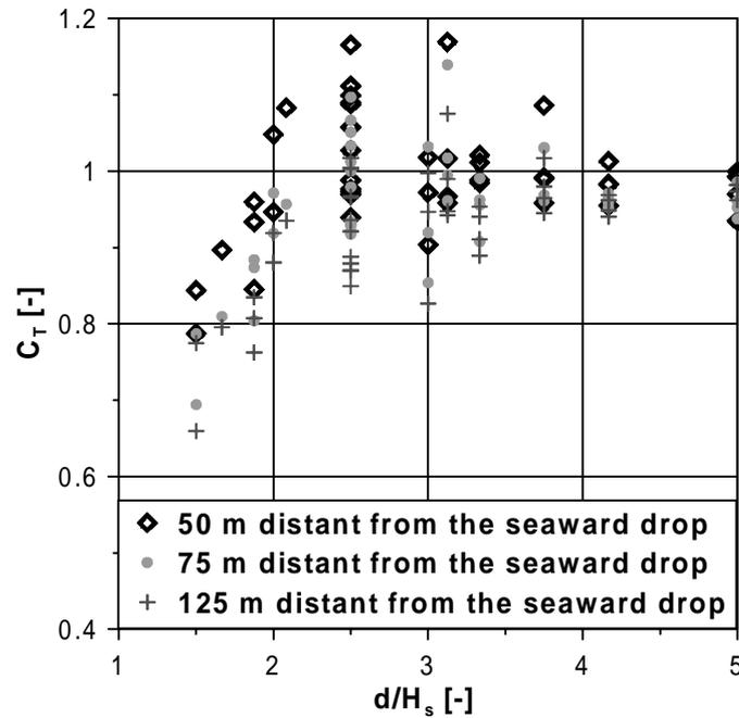
Figure 3: Transmission coefficient  $c_T$  as a function of relative water depth over the foreland at different distances from the seaward drop (derived from experiments in a wave tank)
