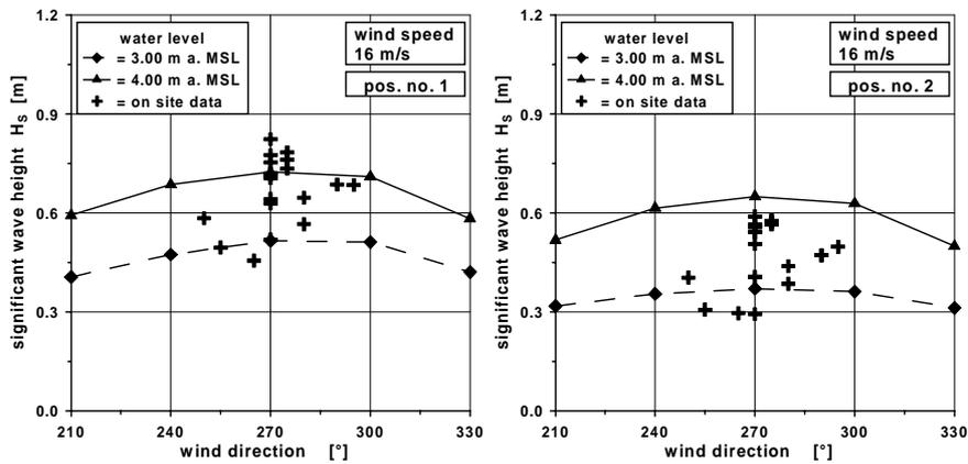
Figure 6: Significant wave height from measurements and SWAN-simulations at pos. no. 1 (left) and pos. 2 (right) (water level: 3 to 4 m a. MSL, wind: 16 m/s, 210° to 330°)
