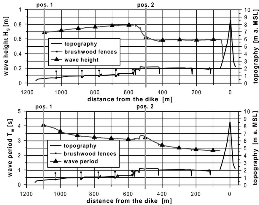
Figure 5: Wave parameter over a foreland at the coast of Dithmarschen – significant wave height (top) and mean wave period (bottom) (water level: 3.8 m a. MSL, wind: 20 m/s, 300°)
