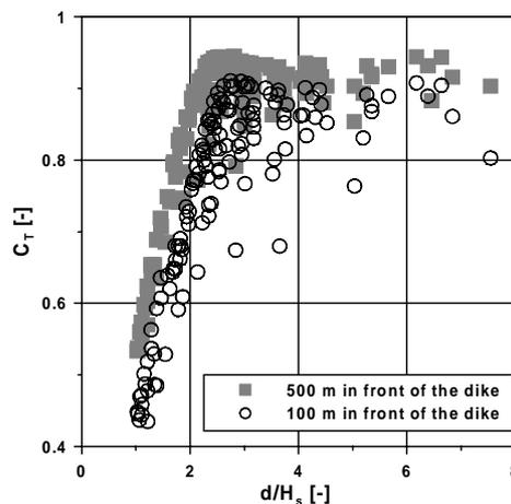
Figure 7: Transmission coefficient as a function of relative water depth at different locations in front of the dike (derived with SWAN)
