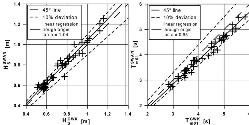
Figure 2: Comparison of physical and numerical modelling of wave propagation along a 125 m wide foreland – significant wave height (left) and mean wave period (right)
