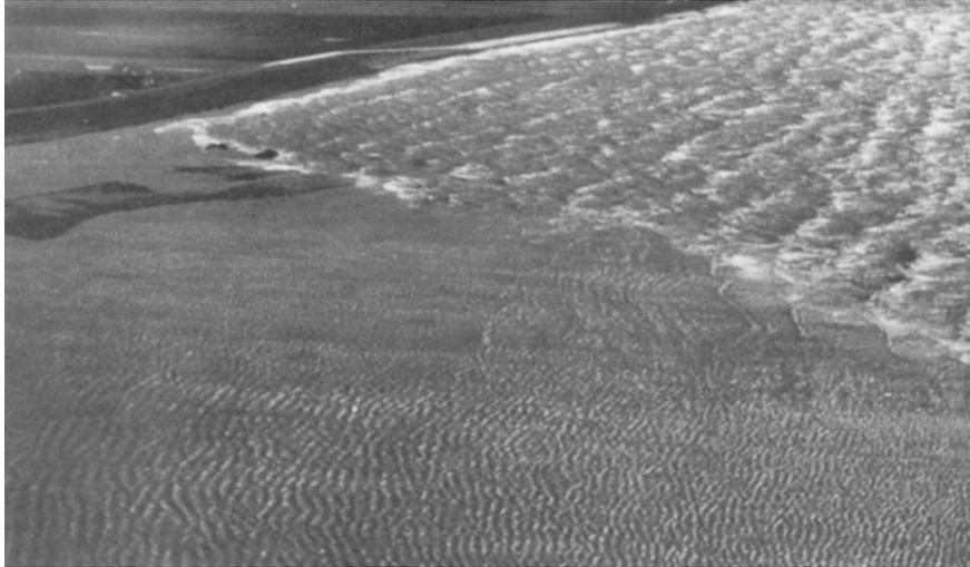
Figure 1: Wave field in front of a dike with (left) and without (right) a foreland.
